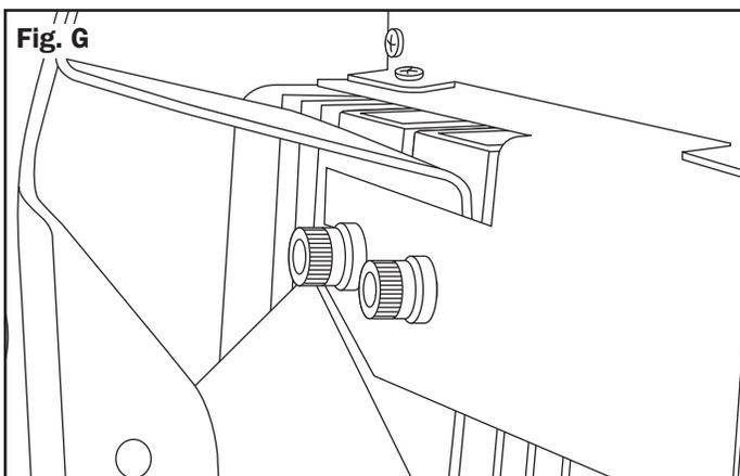
11. Position the J&M Amp/Bracket assembly above the radio and slide into position. (Remove tie-straps and re-position the factory wiring harness as needed to allow the amplifier to fit into place properly)
