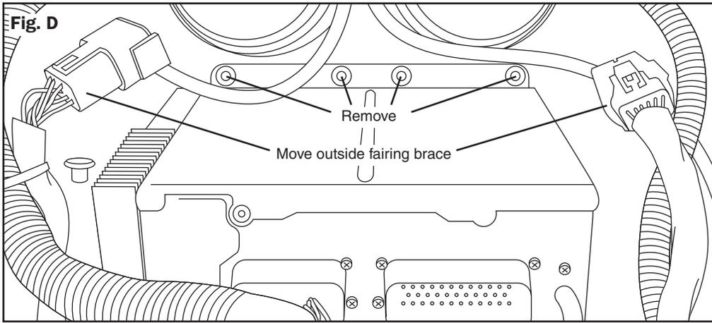
7. Relocate the large plugs from the inside of the fairing braces to the outside of the fairing braces. **(Figure D)**
