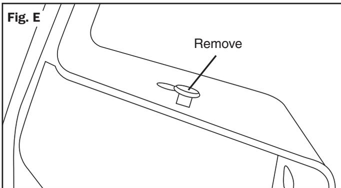
9. Remove the metal stud from the right side fairing brace with a rotary cutting tool. **(Figure E)**
