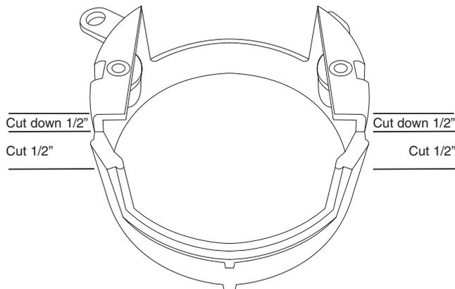
10. Remove the speedometer and tachometer retaining cups and cut out 1/2" of material on the bottom of the cups to allow clearance for the amplifier to be installed. Reinstall the modified gauge retention cups. **(Figure F)** Note: The amplifier should be installed as far back as possible to avoid interfering with the outer fairing shell.
